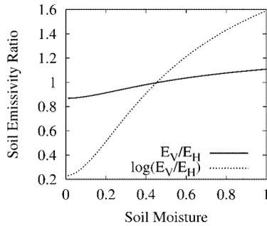
Figure 2. Sensitivity of the simple ratio (normalized by average value)
